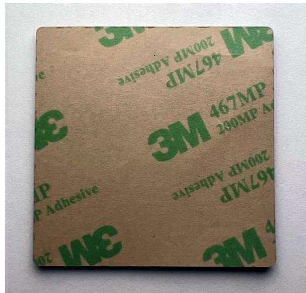
The images above represent top and bottom views of the laser processed ISOLOSS™ LS Polyurethane Foam LS-1506 and 3M™ Adhesive Transfer Tape 467MP with 3M™ Acrylic Adhesive 200MP stack-up. The sample piece demonstrates CO<sub>2</sub> laser cutting (outer edge), kiss-cutting (inner rectangles with top one partially pulled up), engraving (top and bottom text), as well as fiber laser surface marking (logos and DataMatrix code).
